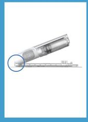
For the micropump to be correctly attached to the infusion assembly, you must engage the notch on the bottom of the micropump with the infusion assembly's hook.
