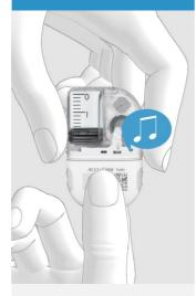
Make sure that there is no gap between the reservoir and the pump base.
