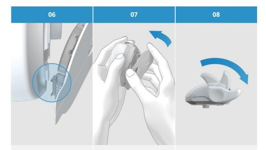
Firstly, align the hook at the bottom of the insertion device and the hook on the pump holder, in such a manner, that they engage with each other. Then, using slight pressure, push the micropump holder all the way onto the insertion device until it engages with the hook on the front of the insertion device. Prime the insertion device by rotating the priming handle clockwise in the direction of the arrow by approx. 180°.
