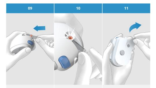
Insert the cannula assembly into the cannula assembly slot in a slanted direction with the lower opening facing forwards. Push the cannula assembly into the slot until you hear it click into place.
