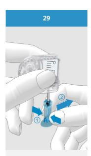
Gently compress the handle aid on the ribbed surface (1) and then remove the handling aid laterally from the piston rod (2).
