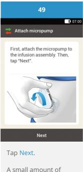
A small amount of insulin is delivered in order to fill the soft Teflon® cannula.
