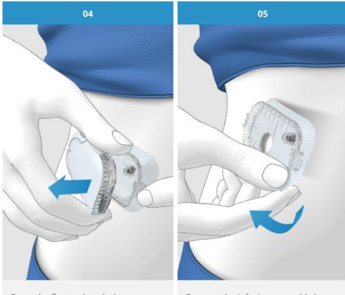
Press the flap to detach the micropump and remove the pump from the infusion assembly. Remove the infusion assembly by loosening the edges of the adhesive pad and then pulling it up and off.
