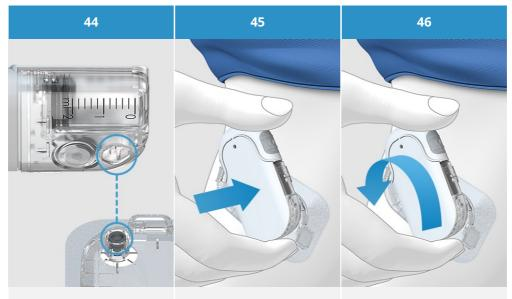
Hold the micropump in a position so that the reservoir needle is above the grey cannula head of the pump holder. Place the reservoir needle of the micropump on the gray cannula head of the pump holder. Turn the micropump carefully in place. You may apply light pressure on the pump shield to make sure the reservoir needle stays inside the cannula head of the pump holder.
