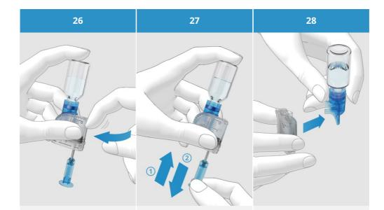
Make sure that there are no air bubbles in the reservoir. Gently tap against the reservoir with your finger to make any air bubbles move in the direction of the filling aid. Slowly push the handle aid upwards in the direction of the arrow (1) to remove air bubbles from the reservoir.
