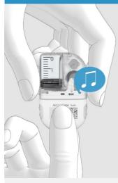
After connecting the reservoir to the pump base, the pumpbase issues 2 beeps to confirm that the system components are correctly connected and the battery is activated. Make sure that there is no gap between the reservoir and the pump base.
