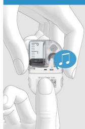
After connecting the reservoir to the pump base, the pumpbase issues 2 beeps to confirm that the system components are correctly connected and the battery is activated.
