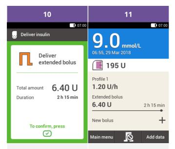
This screen shows you the details of the bolus. Check that they are correct and then press the insulin button to deliver the bolus. The micropump delivers the extended bolus. The display shows the Status screen with a progress bar illustrating the progress of the bolus delivery and the time remaining until completion.
