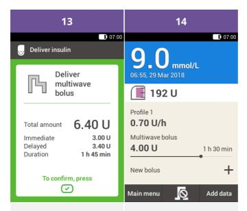
This screen shows you the details of the bolus. Check that they are correct and then press the insulin button to deliver the bolus. The micropump delivers the multiwave bolus. The display shows the Status screen with a progress bar illustrating the progress of the bolus delivery and the remaining time until completion. 7. Delivering a bolus
